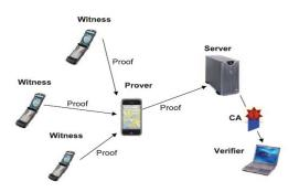
Fig. 1. Location proof updating architecture and message flow.
